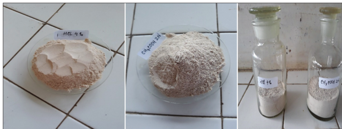
Figure 1: Extract of chicken eggshell from maceration of 4% HCl and CH 3 COOH 2 N
